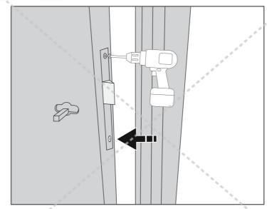
Install the handles on both sides of the lock and finally tighten the bottom with screws.
