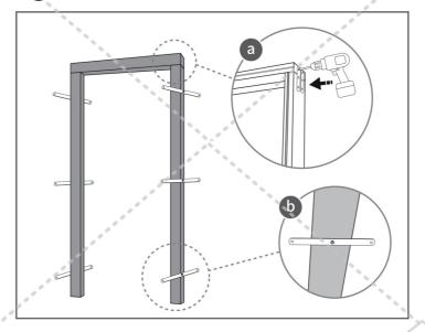
Install the door frame and use the level to check whether both sides are vertical.
