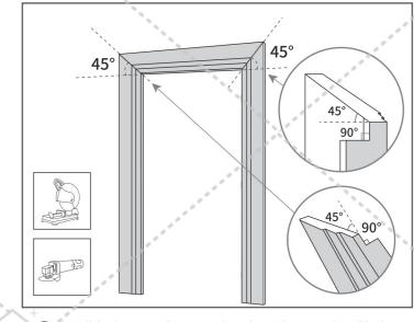
Install the door cover line, spray glass glue at the seams, install both sides of the door cover line first, and then install the top door cover line.
