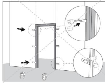
Spray foam, the gap around the inside and outside need to spray foam.
