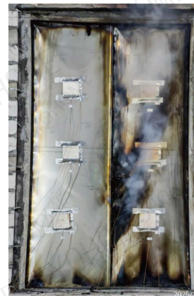
Unexposed Side after 92 Minutes
