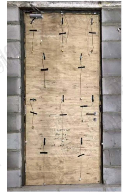
Fig. 2 Unexposed Side Prior to the Fire Test 1
