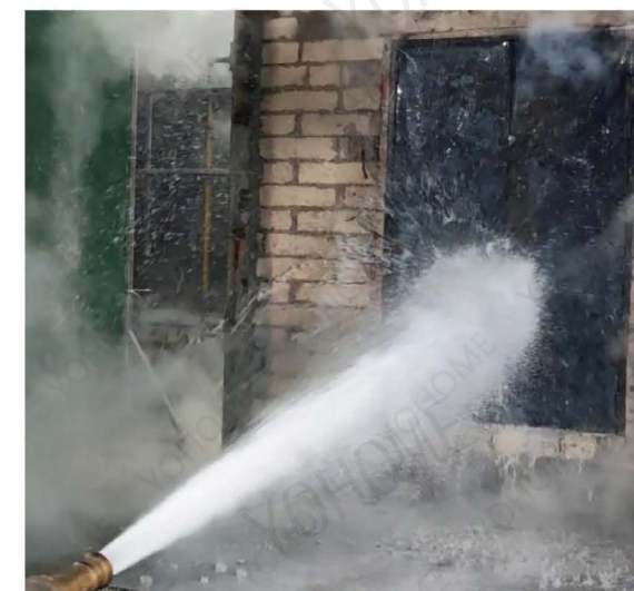
Exposed Side during Hose Stream Test
