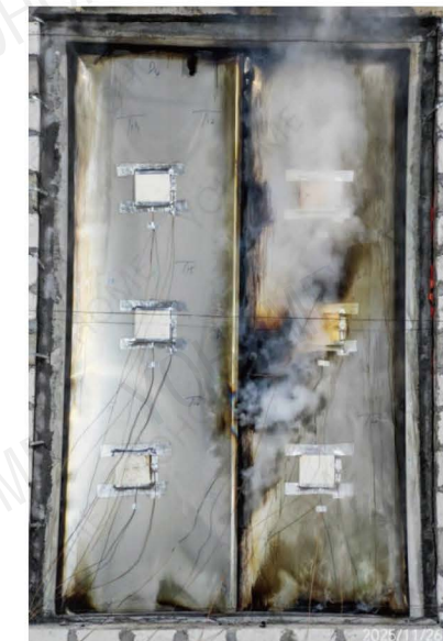
Unexposed Side after 60 Minutes
