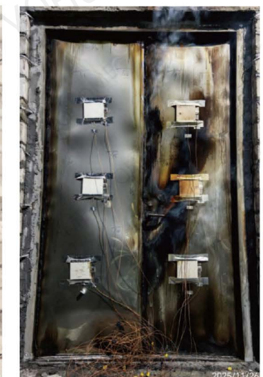
Unexposed Side after Hose Stream Test
