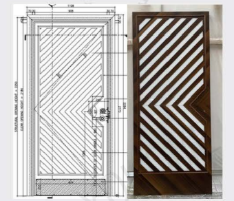
UL 90 min Wooden Fire Door with 38 dB Sound Isolation
