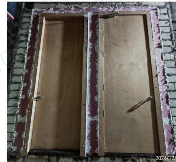
Photo 1 - Exposed Side Prior to the Fire Test
