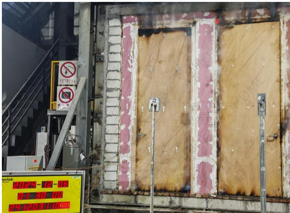
Photo 7 - Unexposed Side after 90 Minutes
