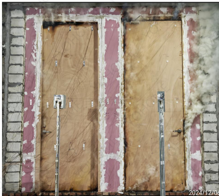
Photo 6 - Unexposed Side after 60 Minutes
