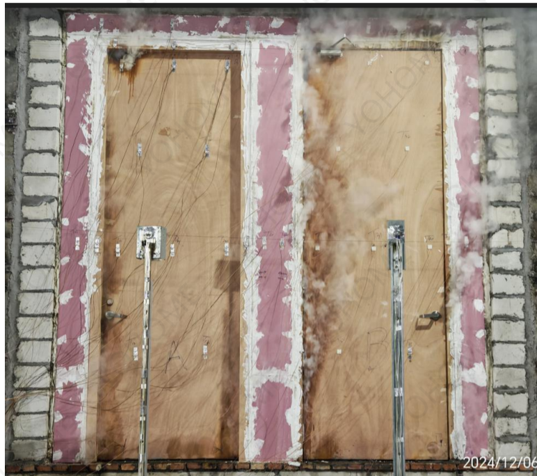
Photo 5 – Unexposed Side after 30 Minutes
