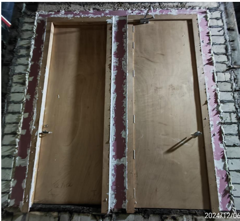
Photo 1 – Exposed Side Prior to the Fire Test
