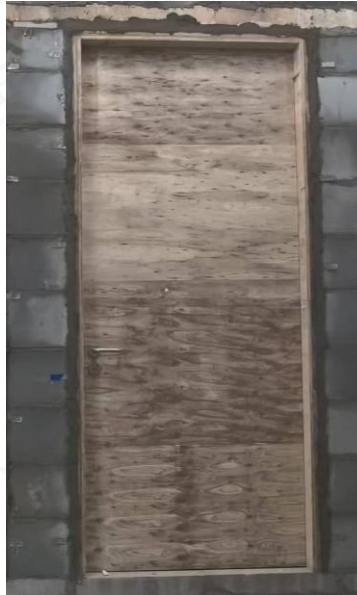
Fig. 1 Exposed Side Prior to the Fire Test 1
