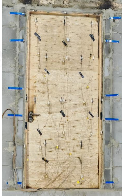
Fig. 11 Unexposed Side after 60 Minutes of the Fire Test 2
