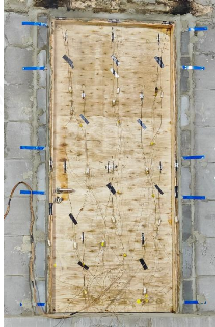
Fig. 9 Unexposed Side after 20 Minutes of the Fire Test 2
