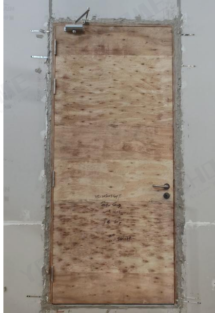
Fig. 13 Unexposed Side of test door assembly before air leakage test 4
