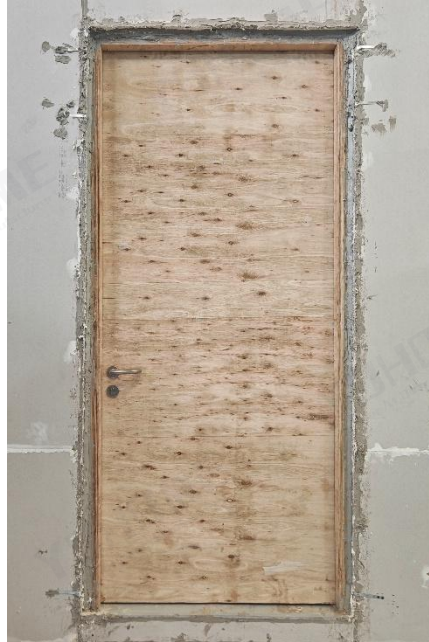
Fig. 17 Unexposed Side of test door assembly before air leakage test 5
