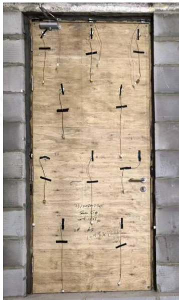
Fig. 2 Unexposed Side Prior to the Fire Test 1
