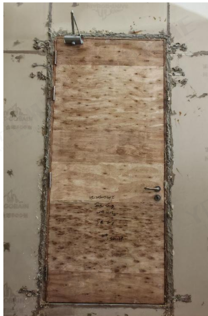
Fig. 18 Exposed Side of test door assembly before air leakage test 5
