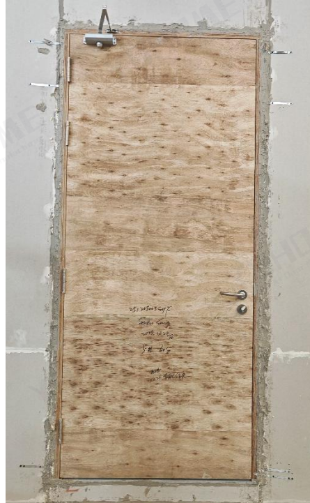
Fig. 15 Unexposed Side of test door assembly after air leakage test 4
