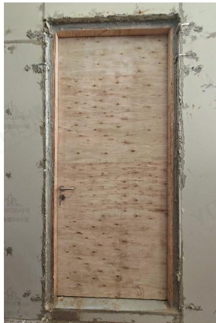
Fig. 14 Exposed Side of test door assembly before air leakage test 4
