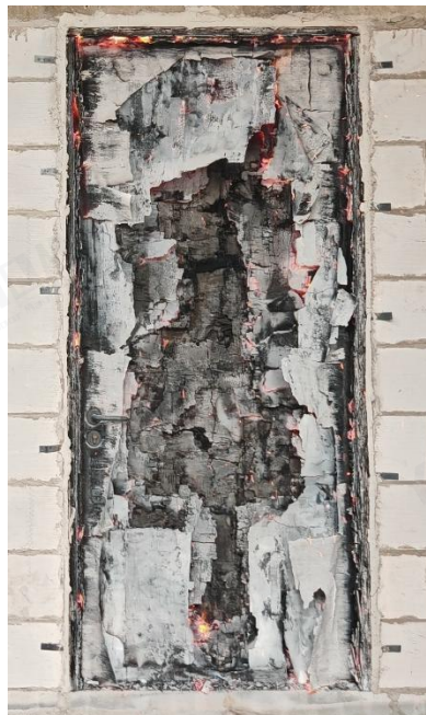
Fig. 6 Exposed Side after 60 Minutes of the Fire Test 1
