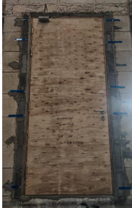
Fig. 7 Exposed Side Prior to the Fire Test 2
