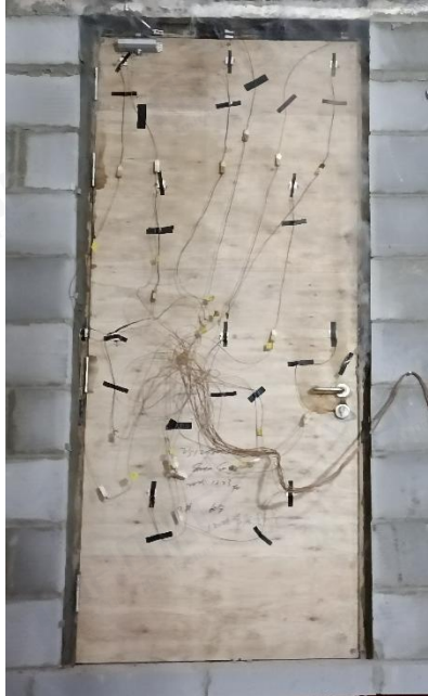
Fig. 3 Unexposed Side after 20 Minutes of the Fire Test 1
