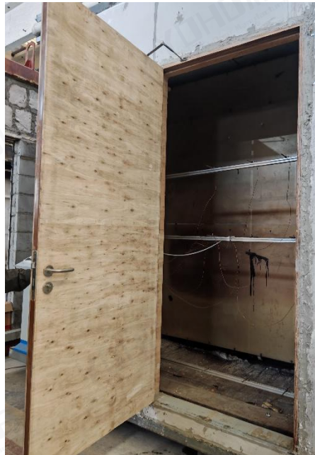
Fig. 16 Exposed Side of test door assembly after air leakage test 4
