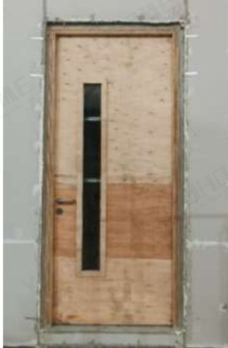
Fig. 9 Unexposed Side of test door assembly before air leakage test 3
