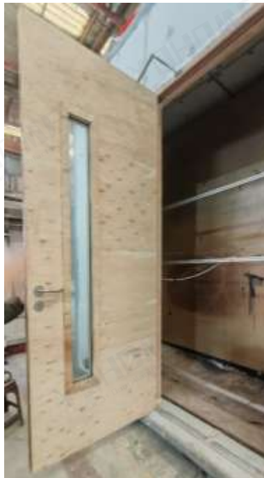
Fig. 8 Exposed Side of test door assembly after air leakage test 2
