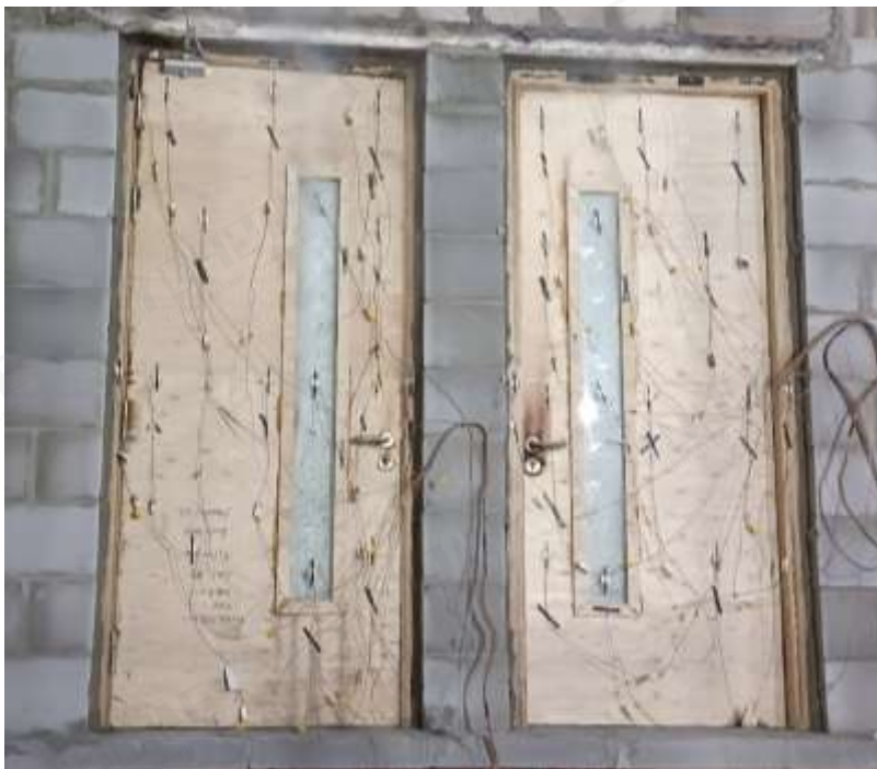
Fig. 4 Unexposed Side after 60 Minutes of the Fire Test 1
