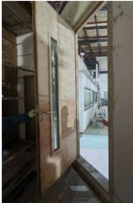
Fig. 10 Test door assembly after air leakage test 3
