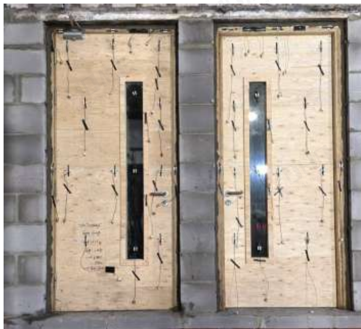
Fig. 2 Unexposed Side Prior to the Fire Test 1
