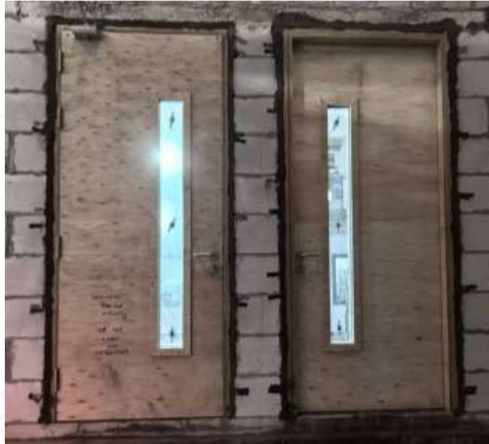
Fig. 1 Exposed Side Prior to the Fire Test 1
