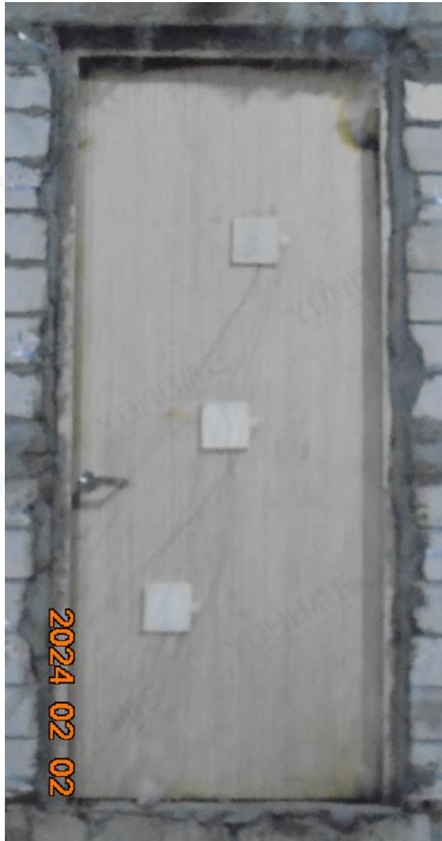
Photo No. 4 Unexposed Side after 20 Minutes
