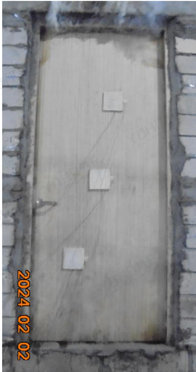
Photo No. 3 Unexposed Side after 10 Minutes
