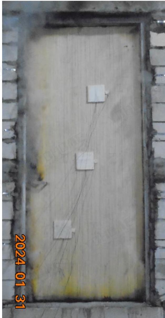
Photo No. 5 Unexposed Side after 45 Minutes
