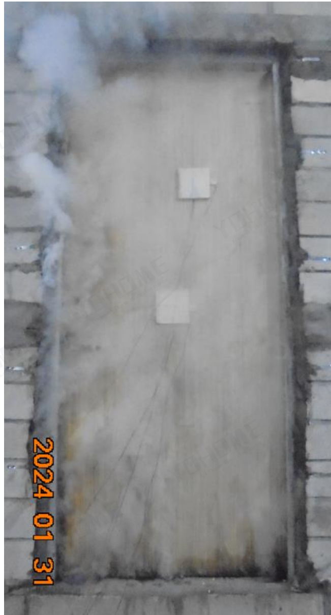
Photo No. 3 Unexposed Side after 15 Minutes
