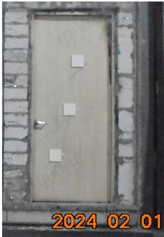
Photo No. 5 Unexposed Side after 60 Minutes
