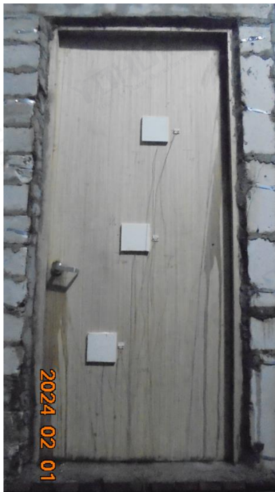
Photo No. 9 Unexposed Side after Hose Stream Test
