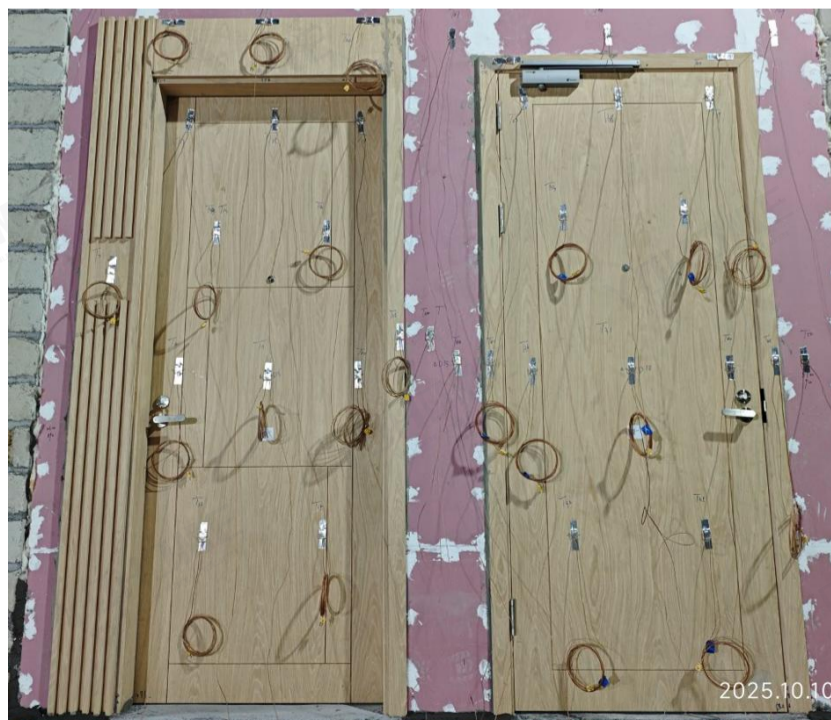
Photo 2 - Unexposed Side Prior to the Fire Test
