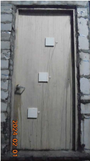
Photo No. 9 Unexposed Side after Hose Stream Test
