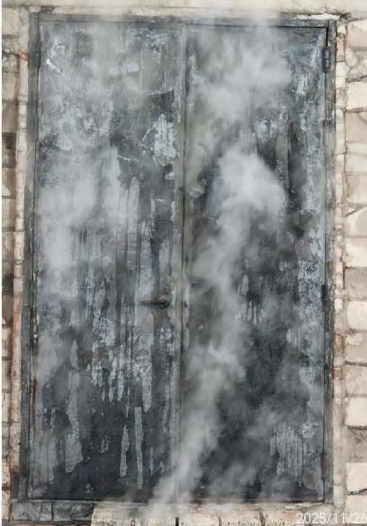
Exposed Side after Hose Stream Test
