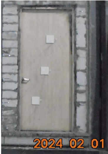
Photo No. 5 Unexposed Side after 60 Minutes
