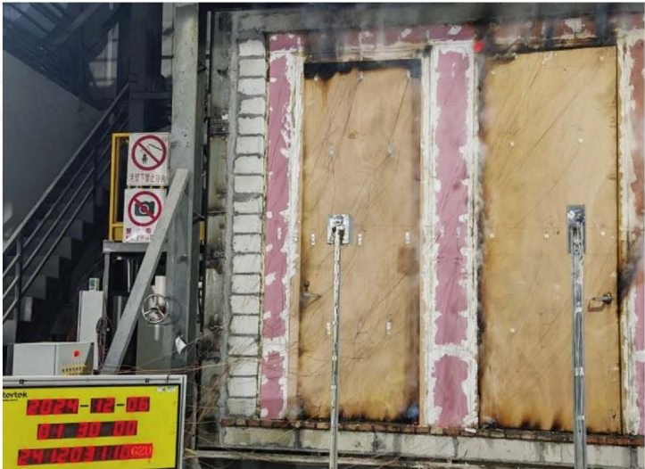
Photo 7 - Unexposed Side after 90 Minutes
