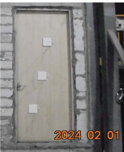
Photo No. 3 Unexposed Side after 20 Minutes
