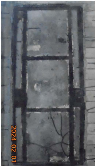
Photo No. 8 Exposed Side after Hose Stream Test
