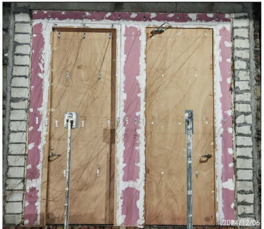
Photo 2 - Unexposed Side Prior to the Fire Test
