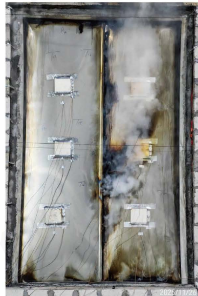
Unexposed Side after 60 Minutes
