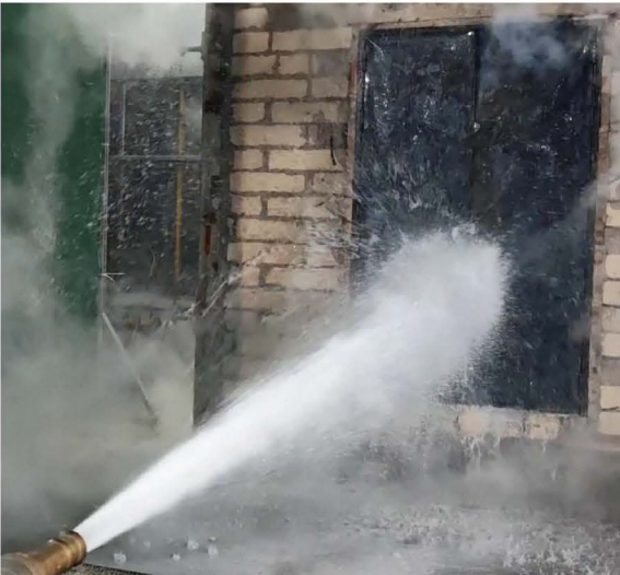
Exposed Side during Hose Stream Test
