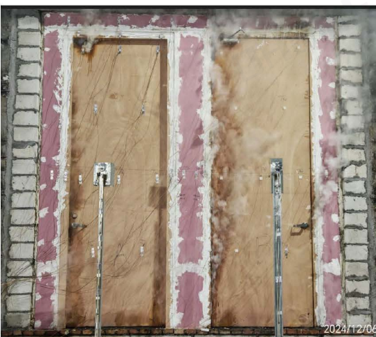
Photo 5 – Unexposed Side after 30 Minutes
