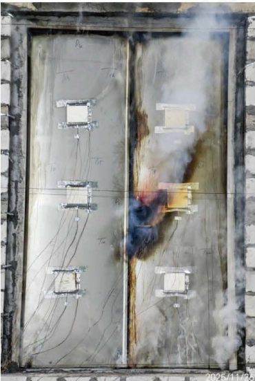
Unexposed Side after 30 Minutes
