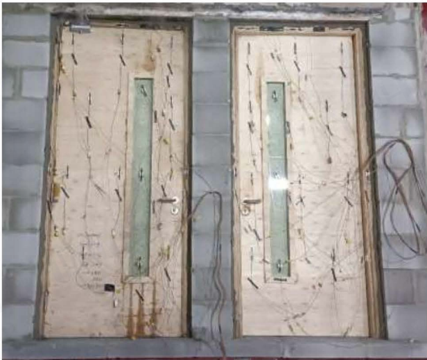
Fig. 3 Unexposed Side after 30 Minutes of the Fire Test 1
