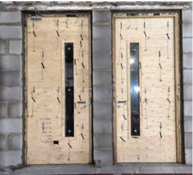
Fig. 2 Unexposed Side Prior to the Fire Test 1
