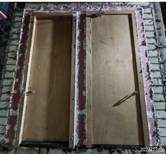
Photo 1 – Exposed Side Prior to the Fire Test
