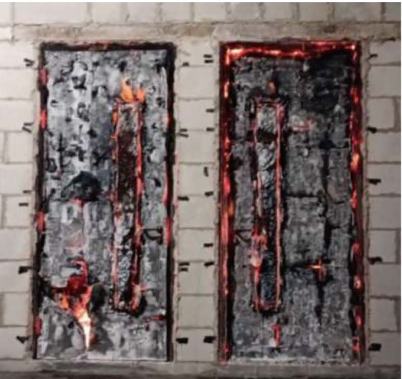
Fig. 6 Exposed Side after 102 Minutes of the Fire Test 1
