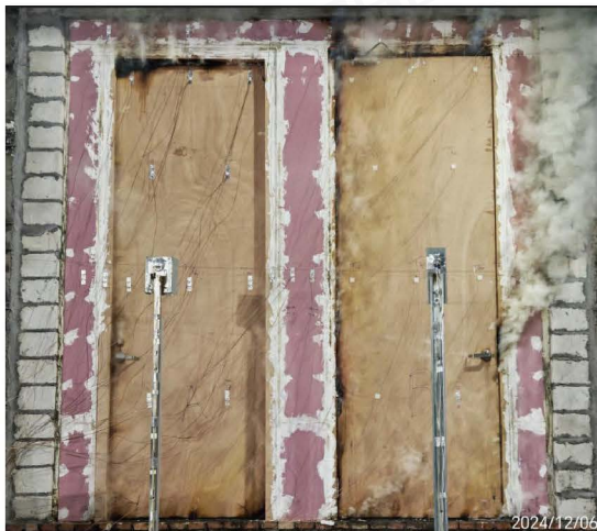
Photo 6 - Unexposed Side after 60 Minutes
