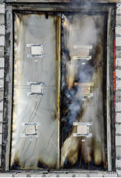
Unexposed Side after 92 Minutes
