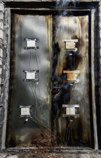
Unexposed Side after Hose Stream Test
